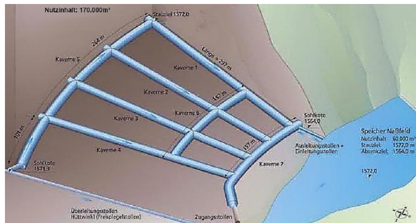
Fig. 1. Planned cavern structure for the extension of the intra-day PSHP plant Nassfeld, Austria [14]
